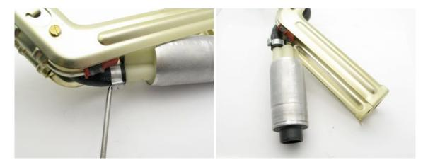
3 – disconnect the electrical connectors and remove the pump from the assembly
