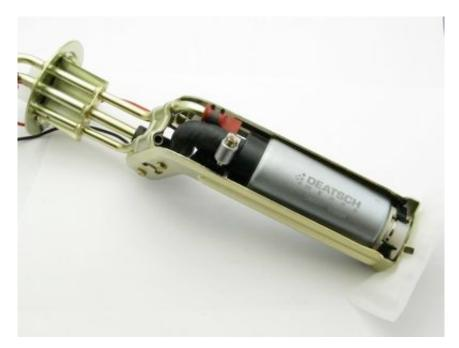
9 – reinstall the assembly into the fuel tank and attach a length of hose to the outlet of the pump assembly allowing it to drain into a fuel safe container and prime the fuel pump assembly
