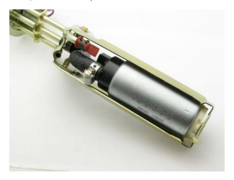
7 – install the fuel sock, retainer clip, and isolator on to the pump
